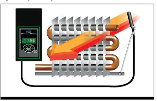
The **coil temperature sensor** provides the input required to determine the current efficiency of the coil and to terminate defrost. It is important that the sensor is located at the coldest point on the coil's surface. This gives the controller the most accurate feedback on the system operating efficiency and helps ensure the coil is completely clear after defrost.
