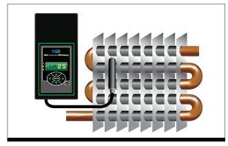
The **suction temperature sensor** is the input used by the controller to calculate the current superheat of the system. This sensor is essential to ensure maximum use of the evaporator's surface area. Maintaining superheat is critical to the safety of the compressor. By having superheat at the exit of the coil, the compressor is certain to be free from liquid floodback.
