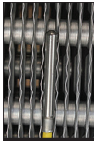
Figure 5 - Option 2: Sensor Positioned Parallel to Evaporator Fins
