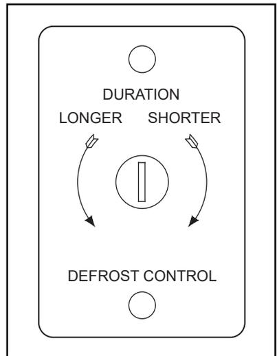
If freezer still remains in defrost too long, a defrost setting pin should be removed from the timer clock. Repeat if necessary.
