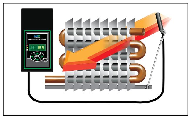
The **coil temperature sensor** provides the input required to determine the current efficiency of the coil and to terminate defrost. It is important that the sensor is located at the coldest point on the coil’s surface. This gives the controller the most accurate feedback on the system operating efficiency and helps ensure the coil is completely clear after defrost.
