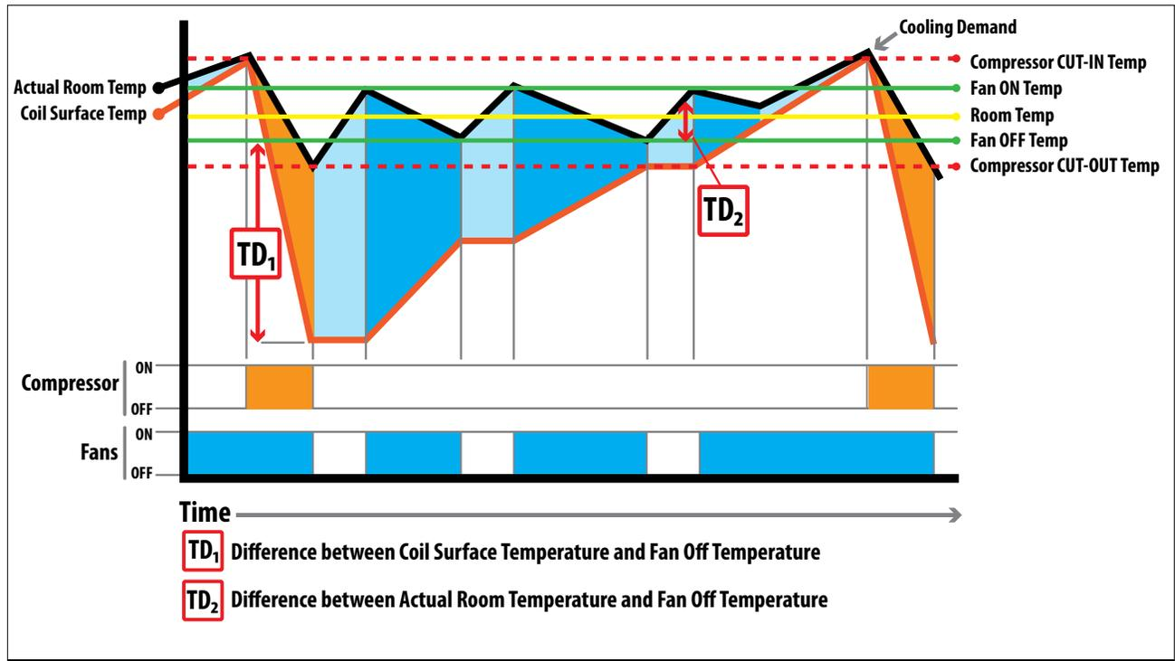
below that of the space temperature, the fans are turned on until the space temperature is satisfied, then turned off. It continues the pattern until the energy stored in the coil is depleted. By continually monitoring the space and coil temperature, the KE2 Evap reduces the frost on the coil. Figure 1 shows how this works in an application.
